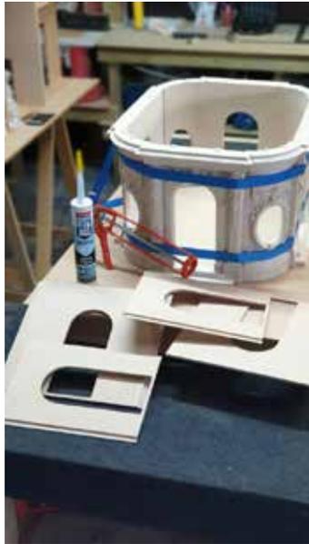
Slice off the domed end of the glue tube but do not slice off the threads otherwise you will not be able to screw on the nozzle. Now screw on the nozzle and slice off the end - the further down the nozzle you slice the bigger the hole. You don't need a large hole so slice near the end of the nozzle.
