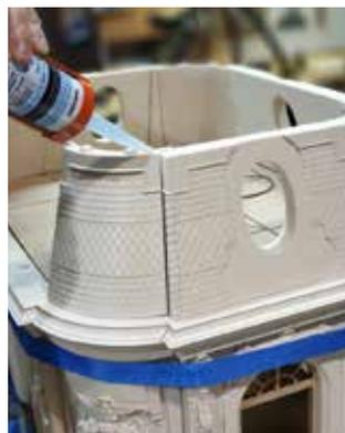
16. Fit roof. Use a mallet if the roof needs a little help
