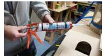
**Preparing your gun:** Push the silver latch towards the trigger and pull the hook away from the trigger.
